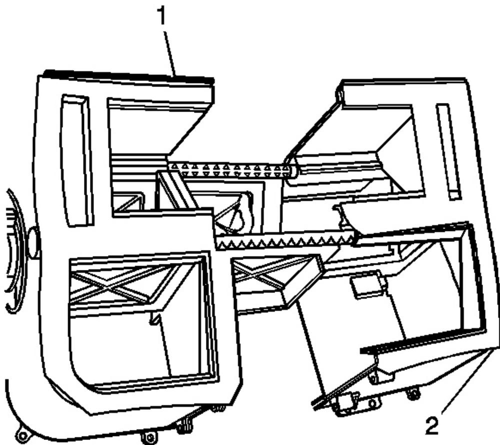
**Fig. 135: Screws & Air Distribution Housing**
