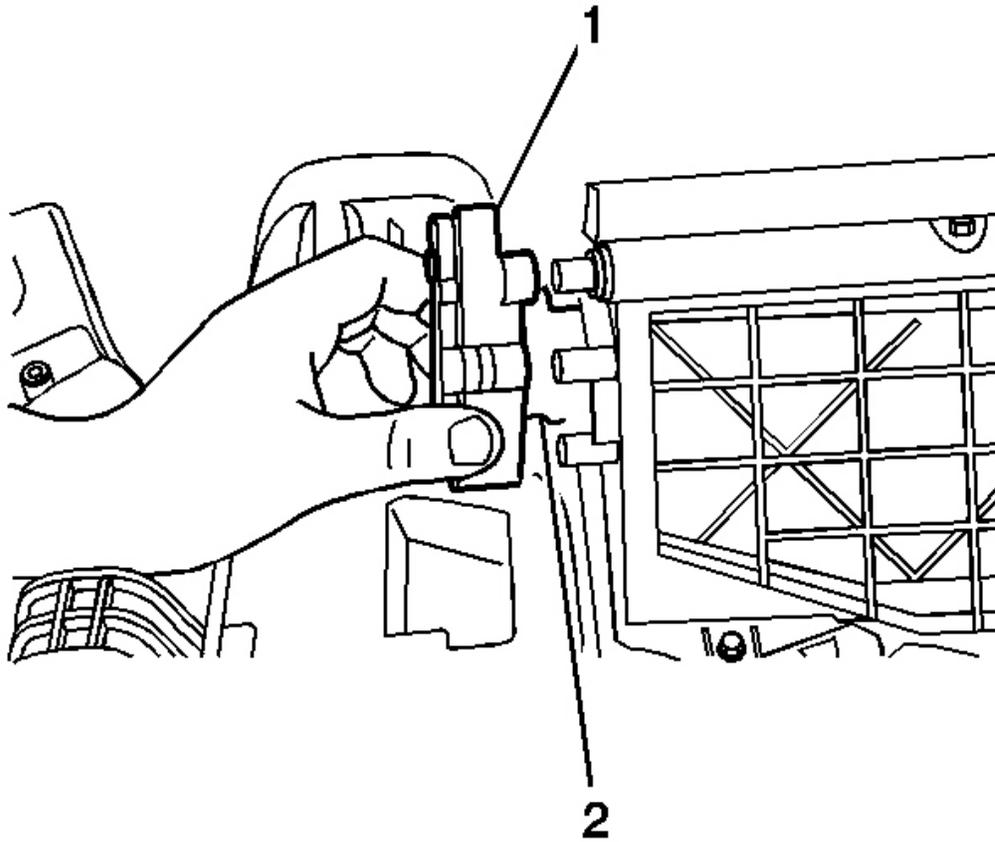
**Fig. 142: Recirculation Actuator And Recirculation Housing**
