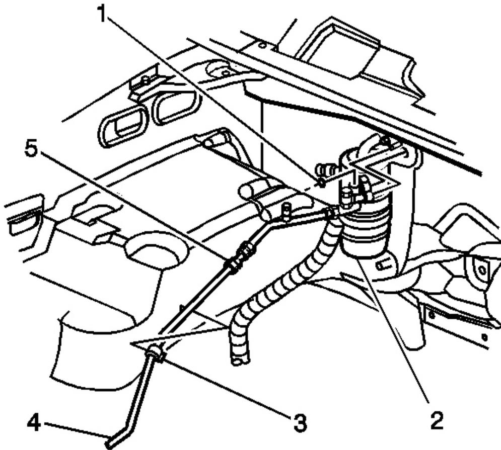
**Fig. 37: A/C Refrigerant Filter & Evaporator Tube**
