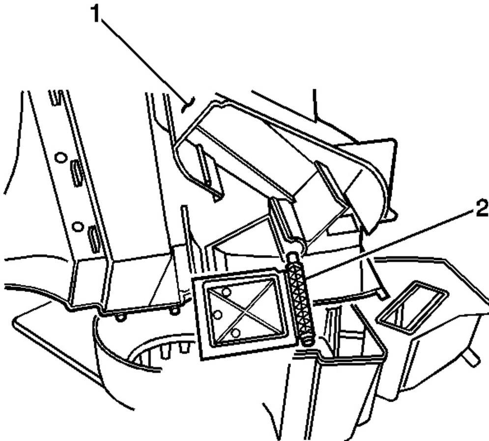
**Fig. 109: Right Temperature Door & Upper HVAC Module Case**
