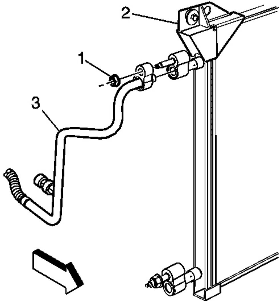
**Fig. 21: Discharge Hose Nut & Condenser**
