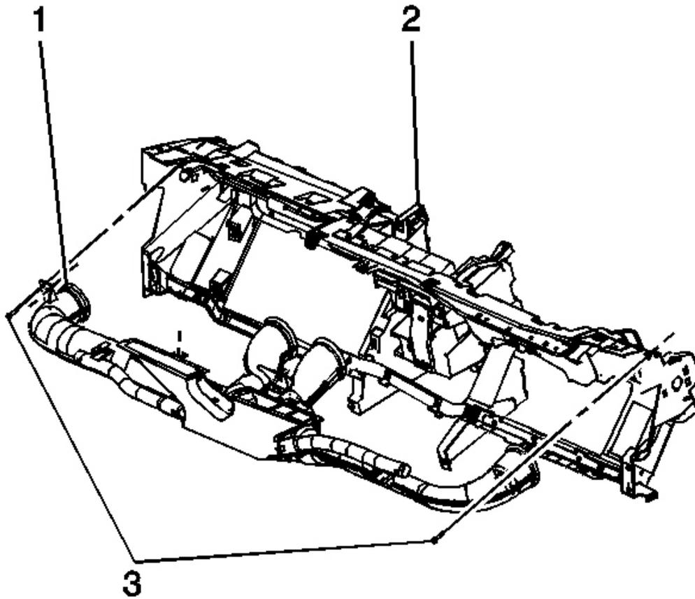
**Fig. 86: Air Distribution Duct & I/P Trim Panel**
