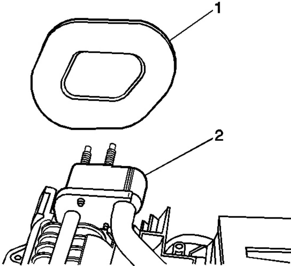
**Fig. 65: Evaporator Cowl Gasket & Evaporator**
