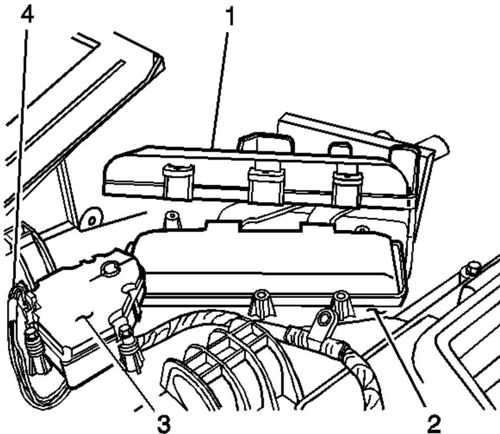
**Fig. 147: Heater Core Cover And HVAC Module Assembly**
