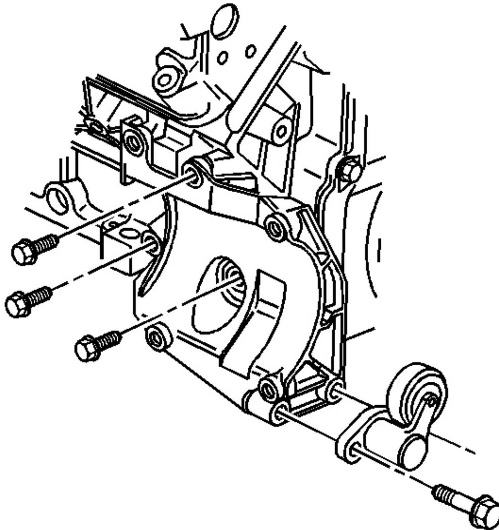
**Fig. 13: A/C Compressor Bracket**
