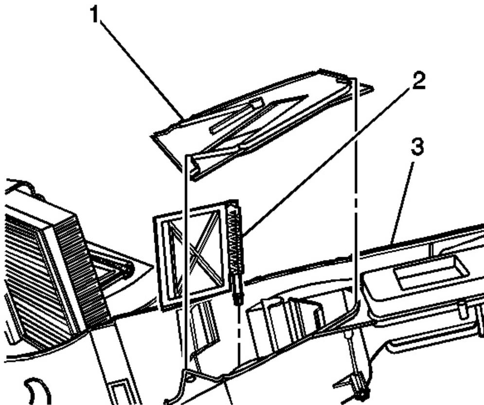
**Fig. 121: Left Temperature Door & Lower HVAC Module Case**
