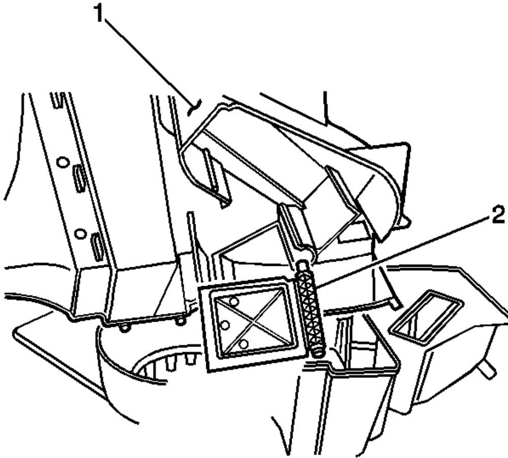
**Fig. 108: Right Temperature Door & Upper HVAC Module Case**
