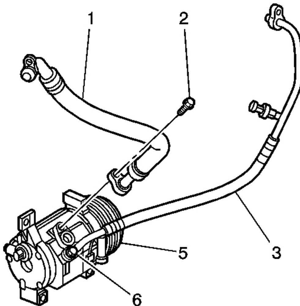
**Fig. 20: Discharge Hose & A/C Compressor**
