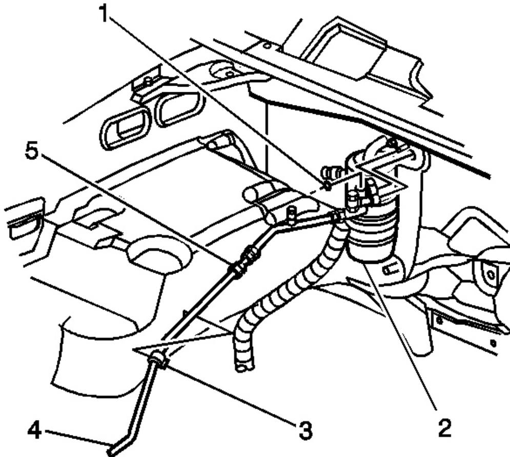
**Fig. 32: A/C Refrigerant Filter & Evaporator Tube**
