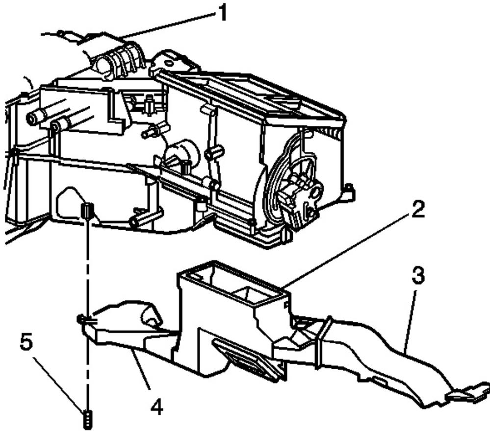
**Fig. 101: Floor Air Outlet Duct (RH)**
