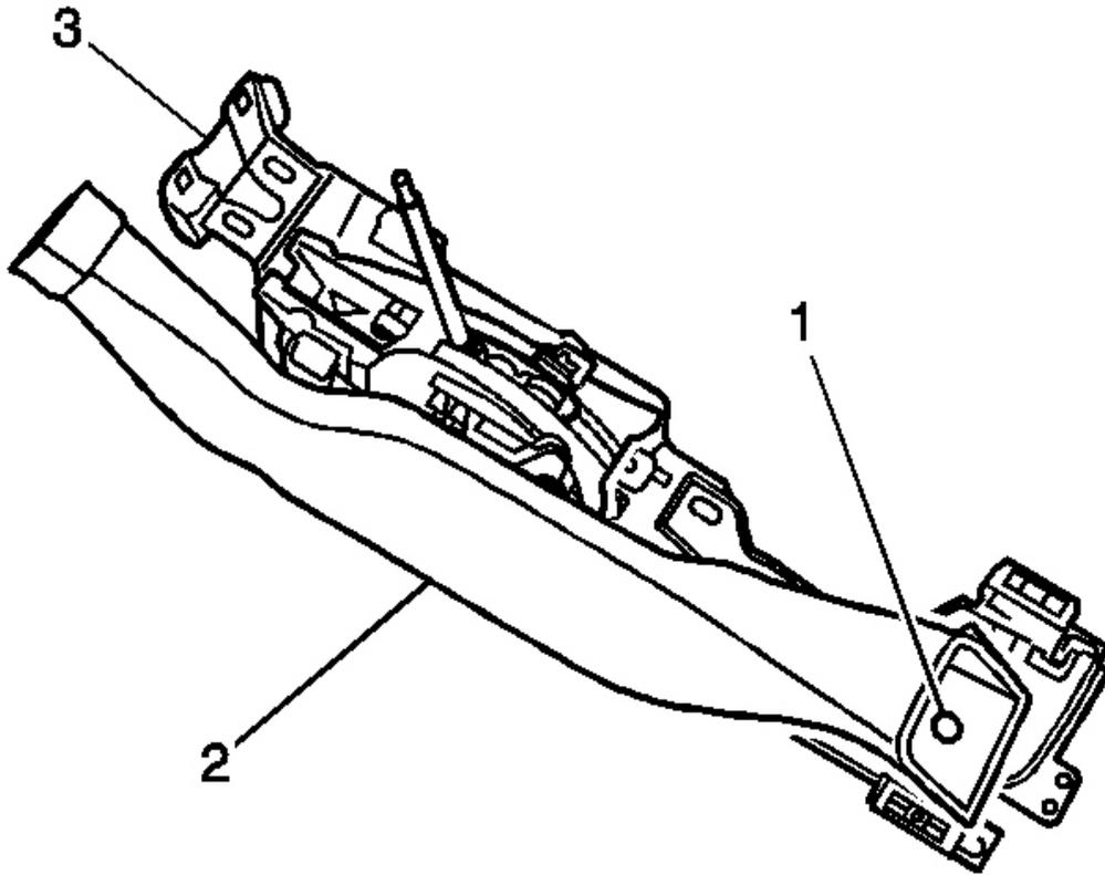
**Fig. 98: Identifying Push Pin (Rear Floor)**
