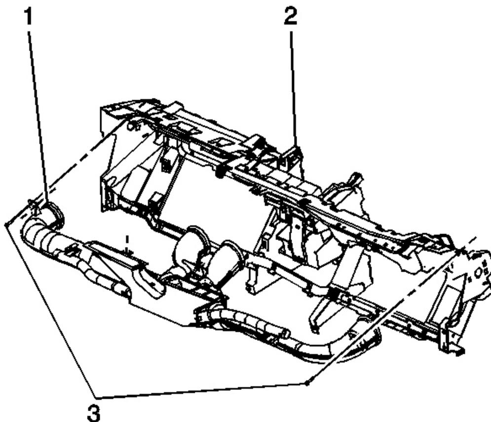
**Fig. 87: Air Distribution Duct & I/P Trim Panel**
