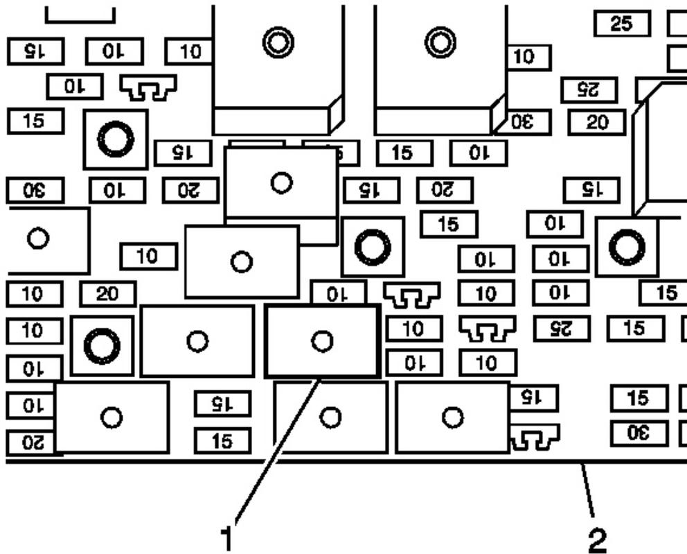
**Fig. 44: A/C Compressor Relay & Convenience Center**
