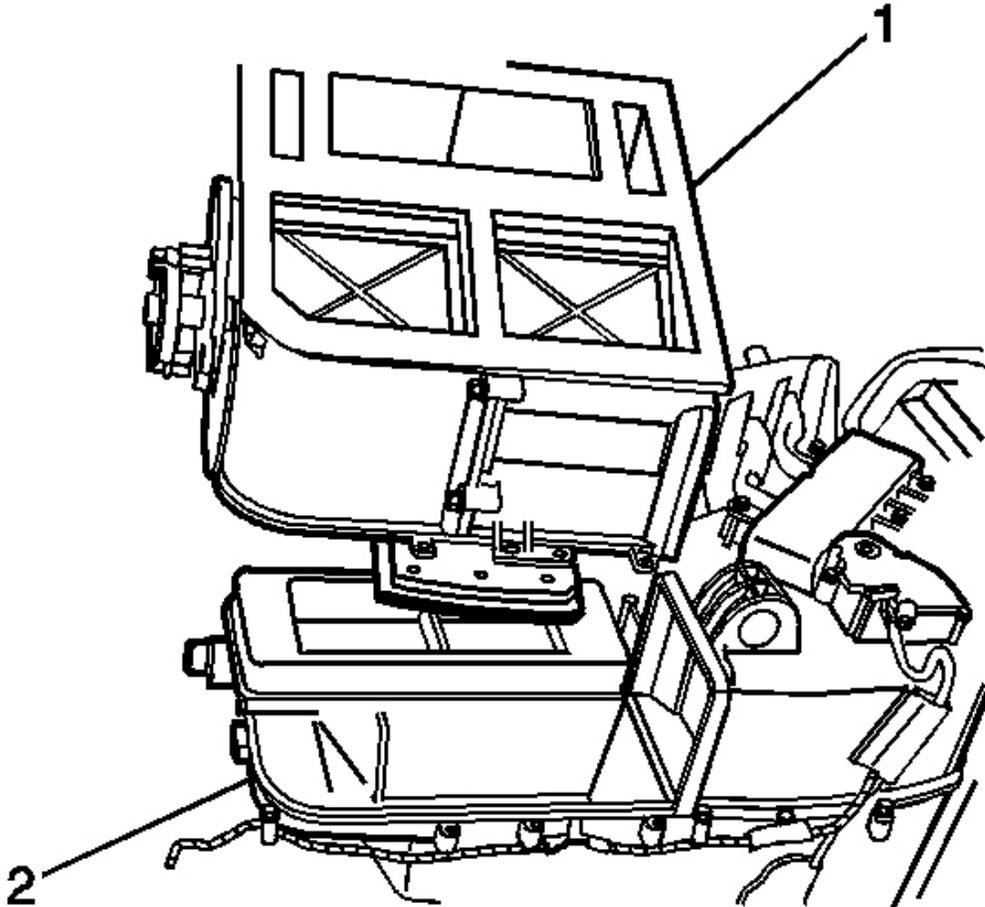
**Fig. 131: Air Distribution Housing And HVAC Module Assembly**
