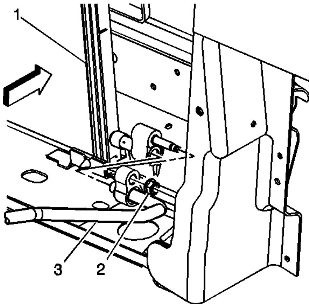
**Fig. 50: Evaporator Tube & Condenser**
