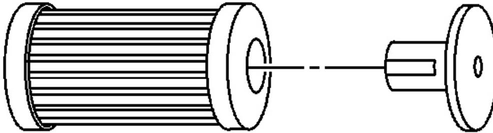
**Fig. 2: Removing Check Valve**
