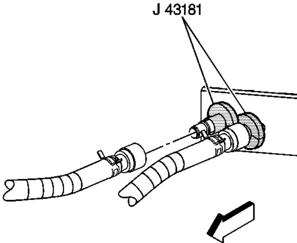
**Fig. 60: Identifying Heater Hose To Heater Core Outlet**
