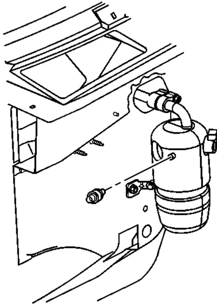
**Fig. 45: A/C Low Pressure Switch & Accumulator**
