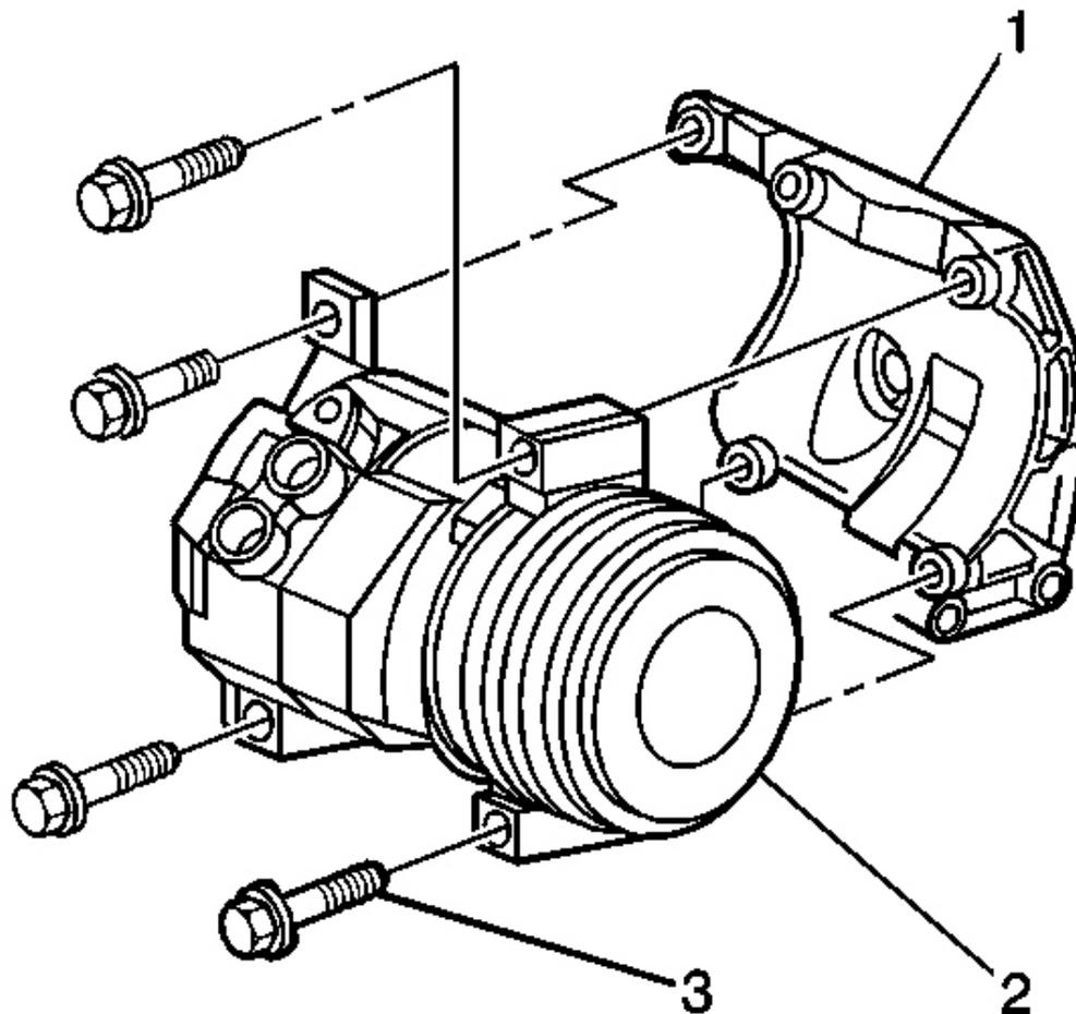
**Fig. 7: A/C Compressor Mounting Bolts (L18)**
