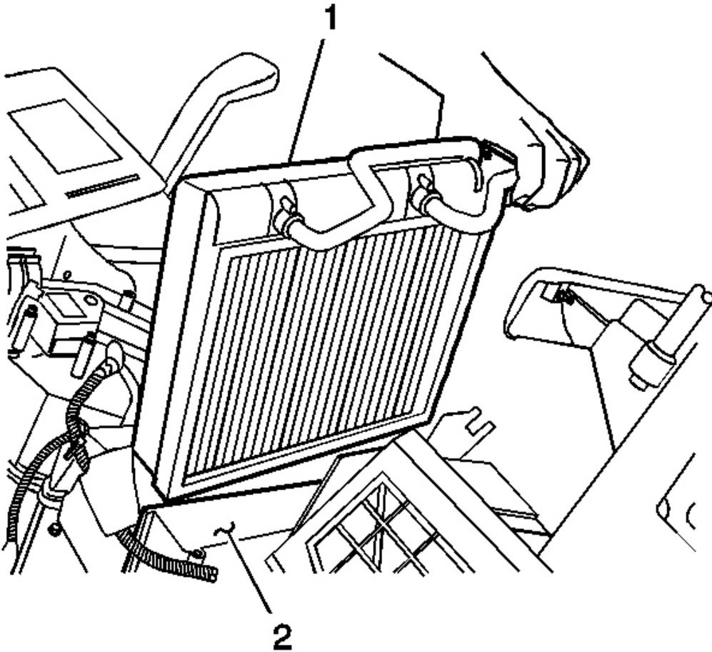
**Fig. 63: Evaporator Core & HVAC Module**
