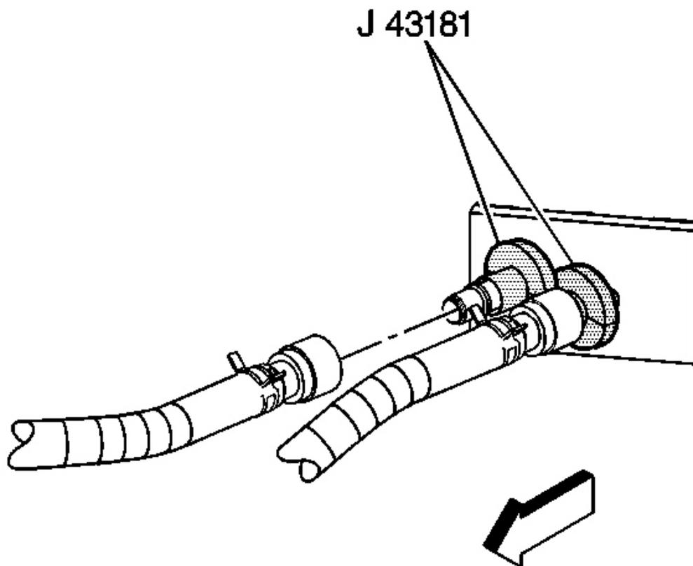
**Fig. 73: Identifying Heater Hose To Heater Core Outlet**
