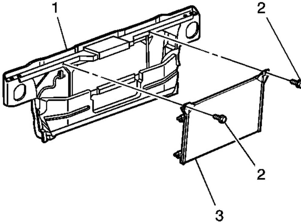
**Fig. 52: Condenser & Mounting Bolts**
