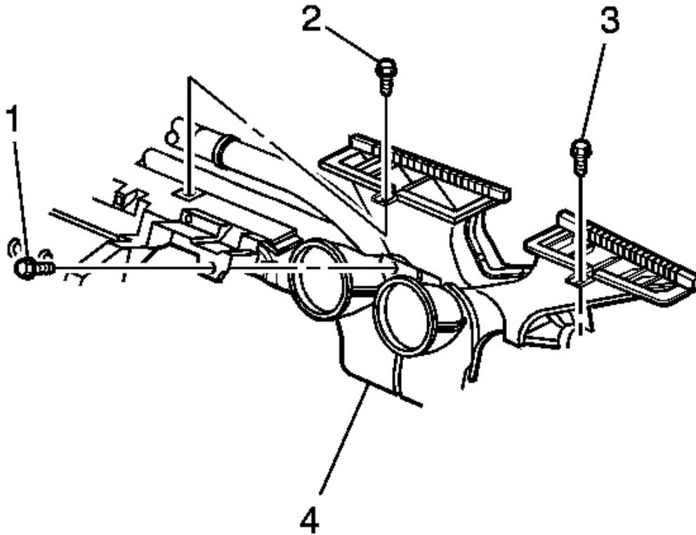
**Fig. 85: Screw & Air Distribution Duct**
