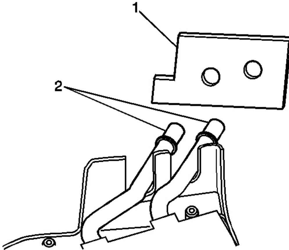
**Fig. 148: Heater Core Cowl Gasket & Heater Core**
