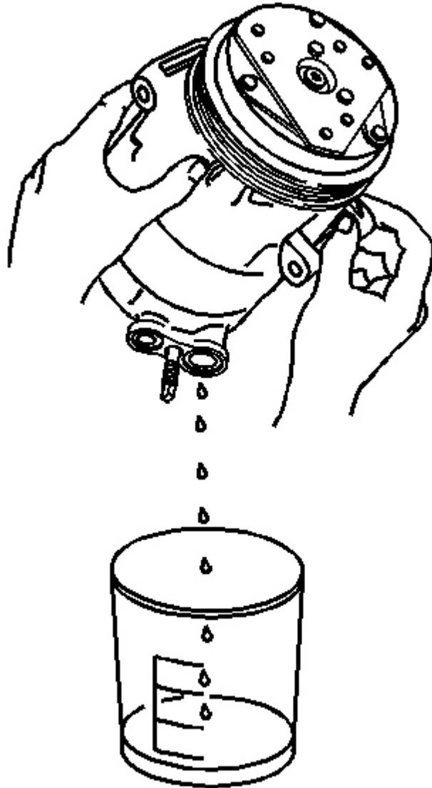
**Fig. 3: Draining A/C Compressor Oil**
