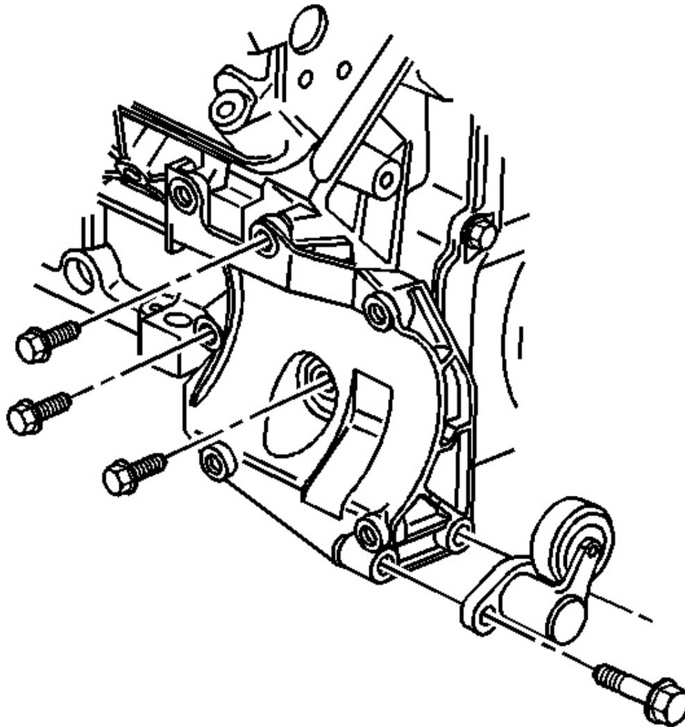
**Fig. 14: A/C Compressor Bracket**
