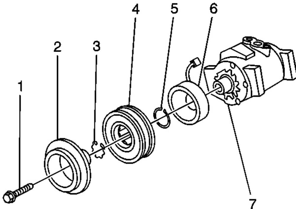
**Fig. 10: Exploded View Of Compressor Clutch Plate Assembly**
