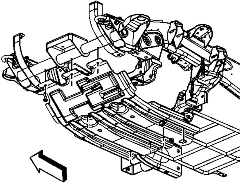
**Fig. 8: Removing Engine Protection Shield**
