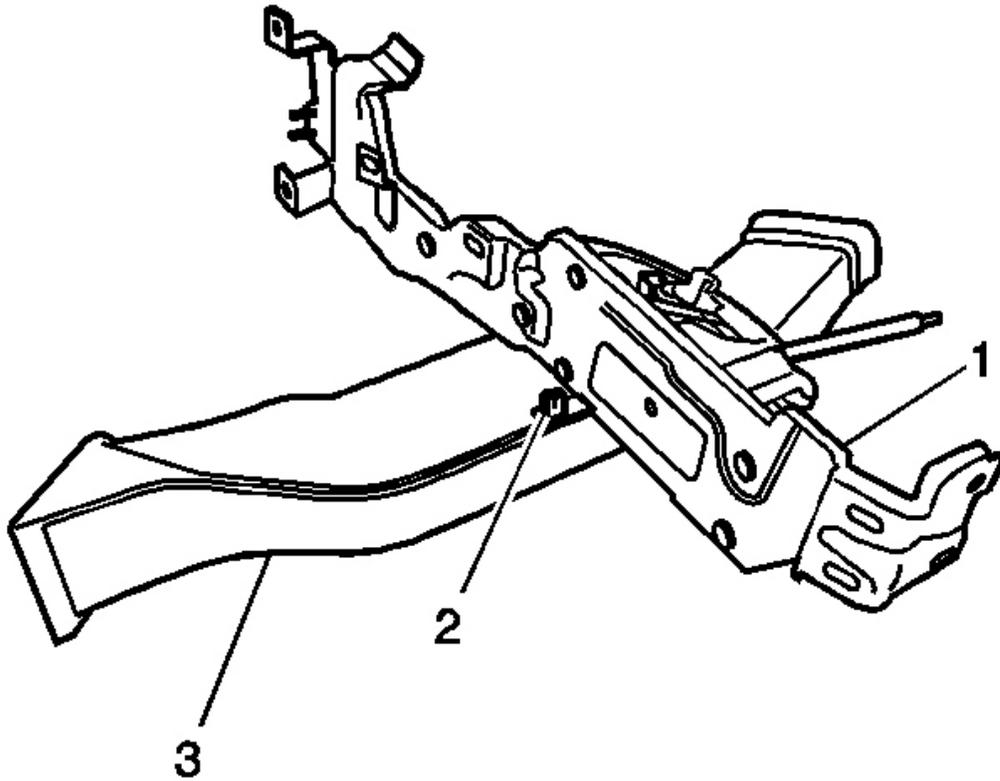
**Fig. 97: Air Outlet Duct & Console Support Bracket (Rear Floor)**
