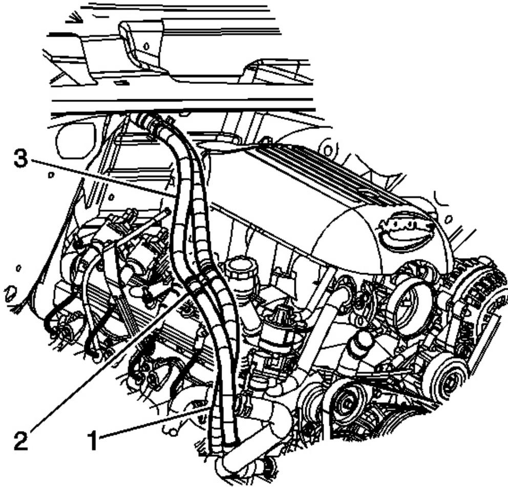
**Fig. 71: Heater Inlet Hose & Mounting Clip**
