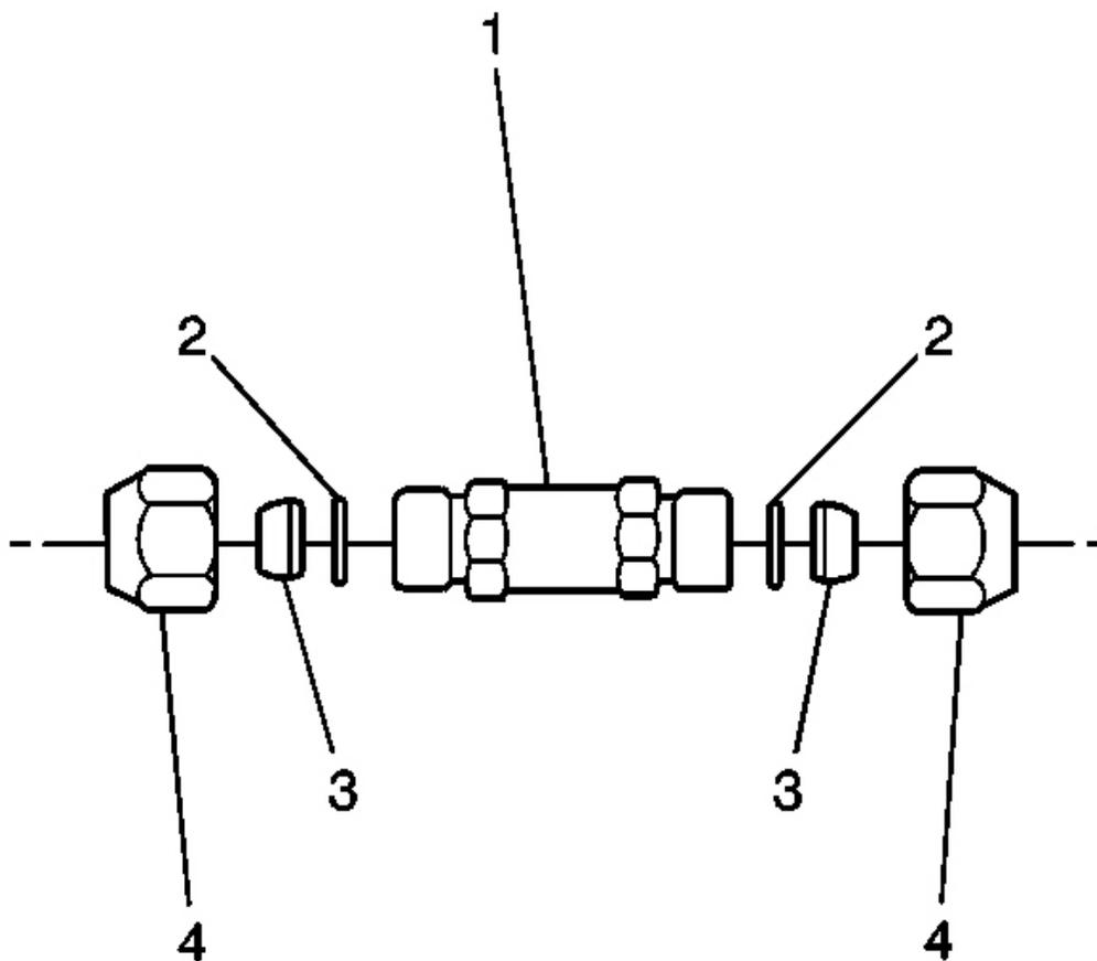
**Fig. 40: A/C Refrigerant Filter Components**
