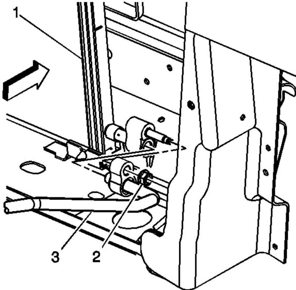
**Fig. 28: Evaporator Tube & Condenser**
