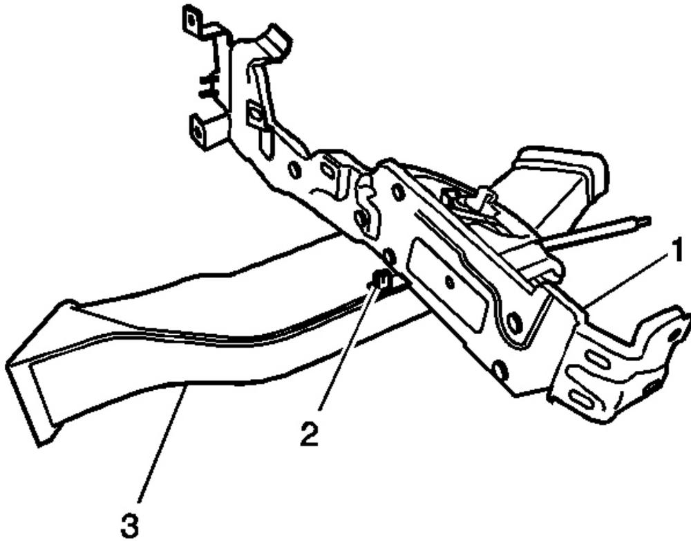
**Fig. 96: Air Outlet Duct & Console Support Bracket (Rear Floor)**
