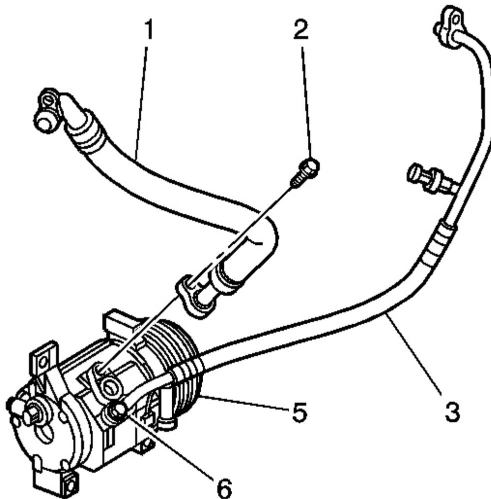
**Fig. 24: Discharge Hose & A/C Compressor**
