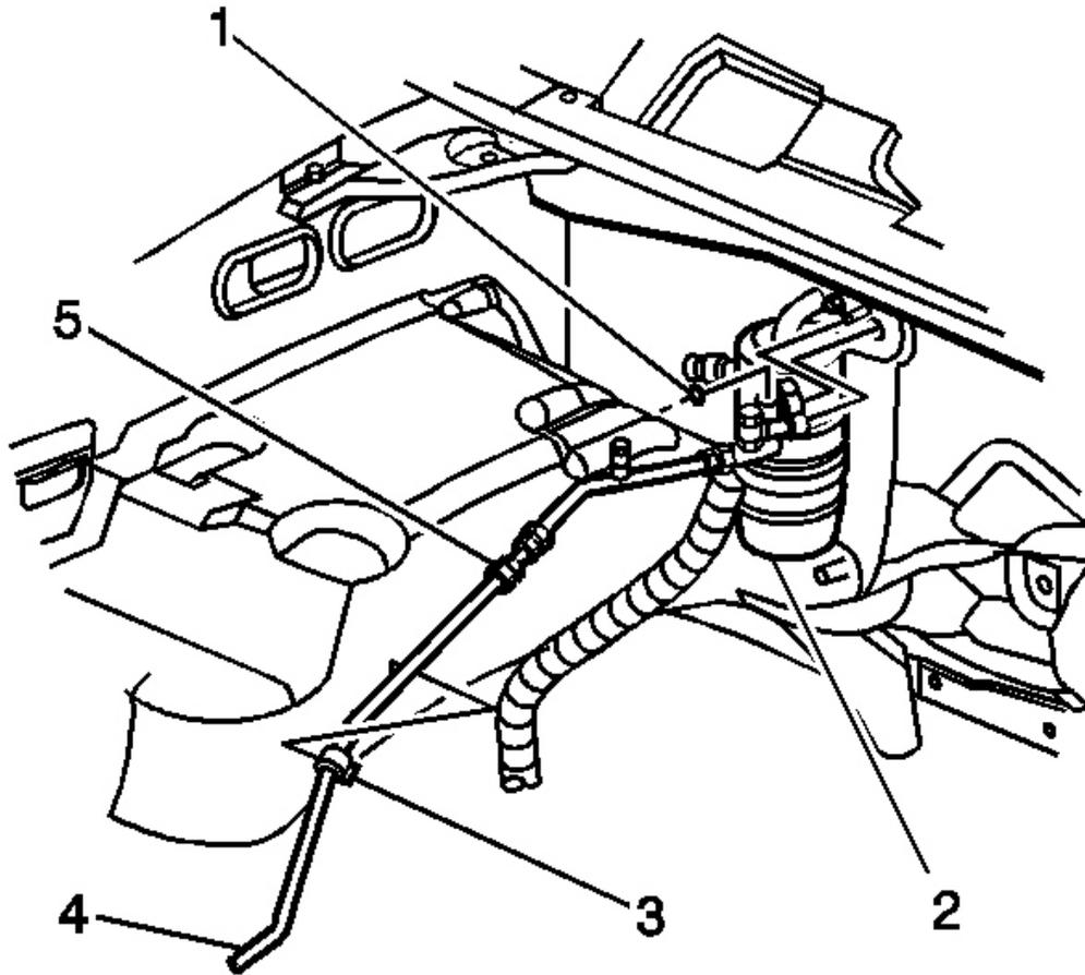
**Fig. 34: A/C Refrigerant Filter & Evaporator Tube**
