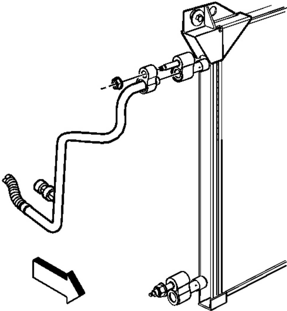
**Fig. 47: A/C Refrigerant Pressure Sensor & Evaporator Tube**
