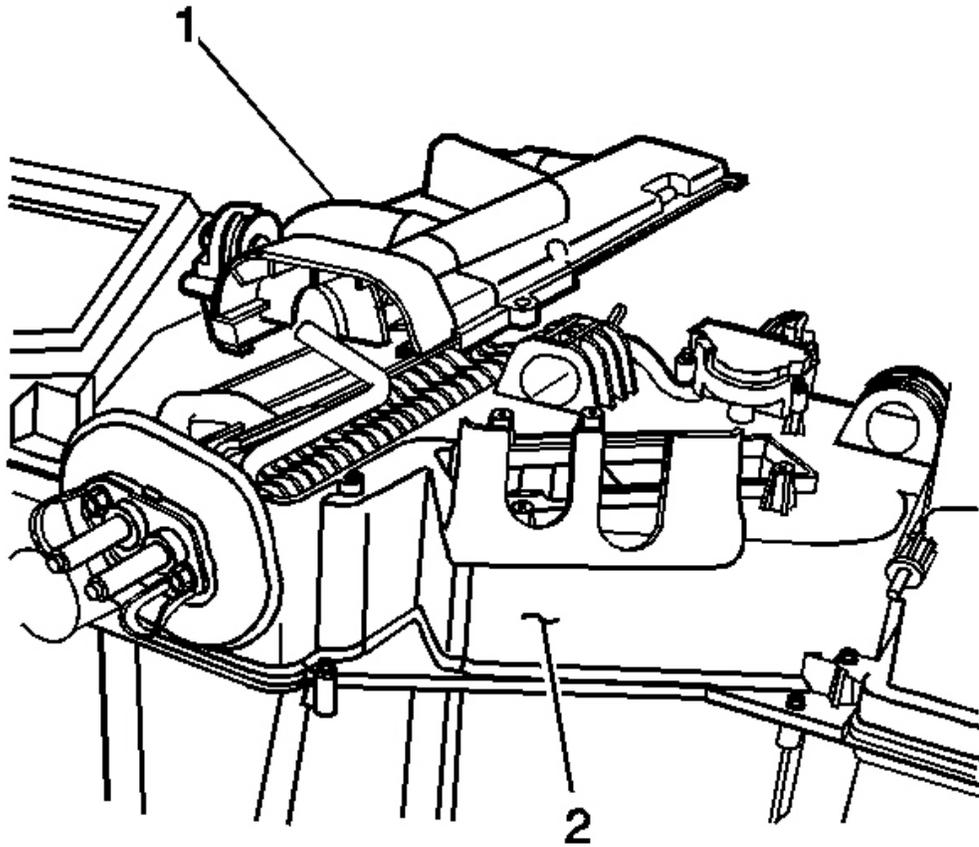
**Fig. 61: Evaporator Cover & HVAC Module**
