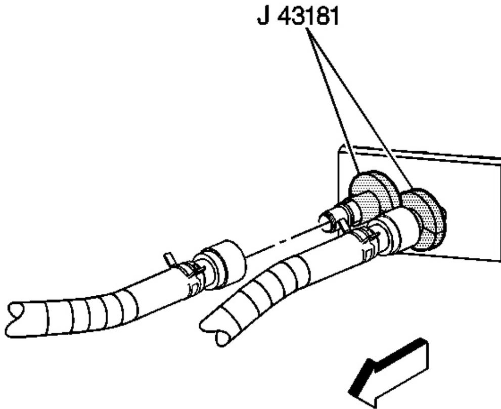
**Fig. 72: Identifying Heater Hose To Heater Core Outlet**
