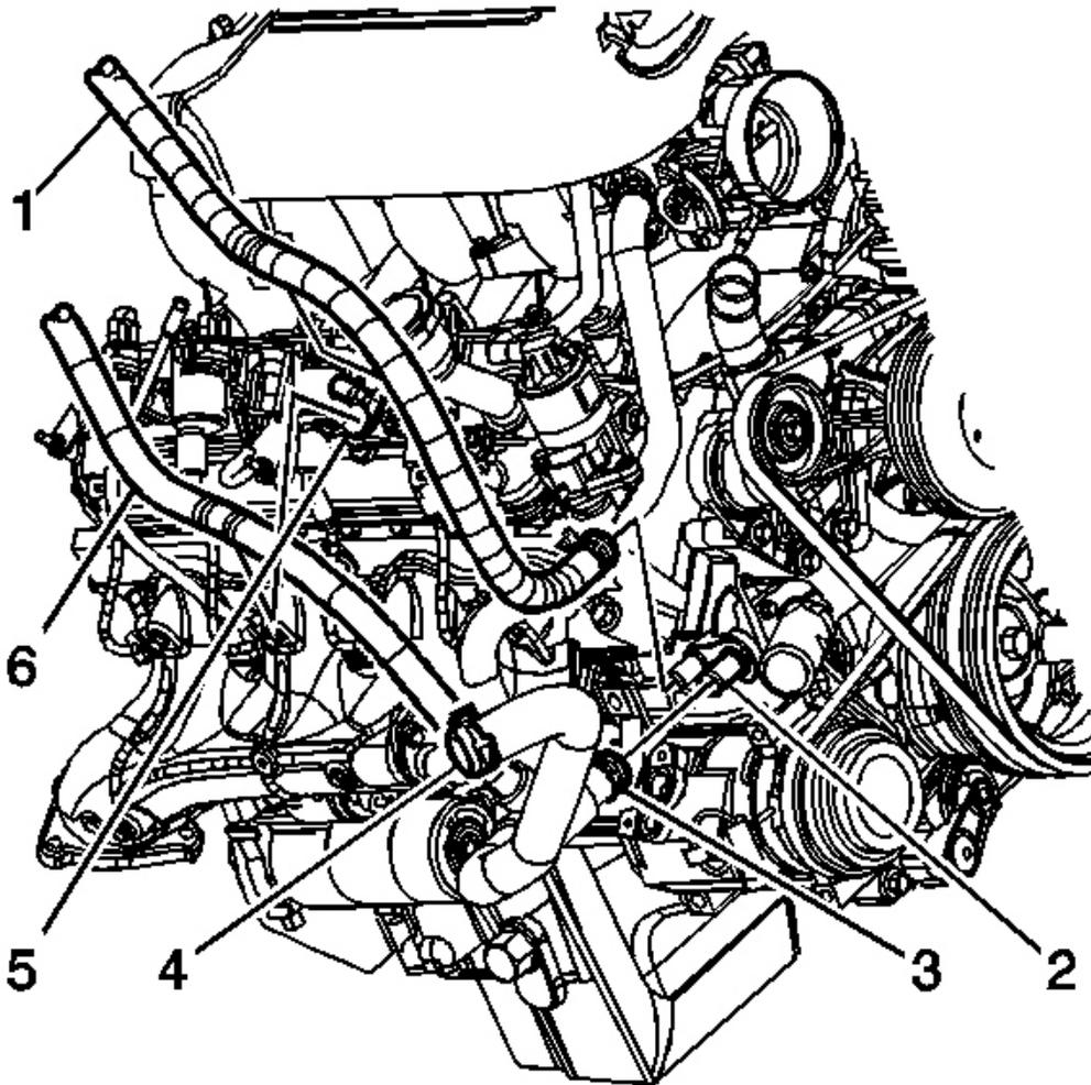
**Fig. 78: Heater Inlet Hose & Engine**
