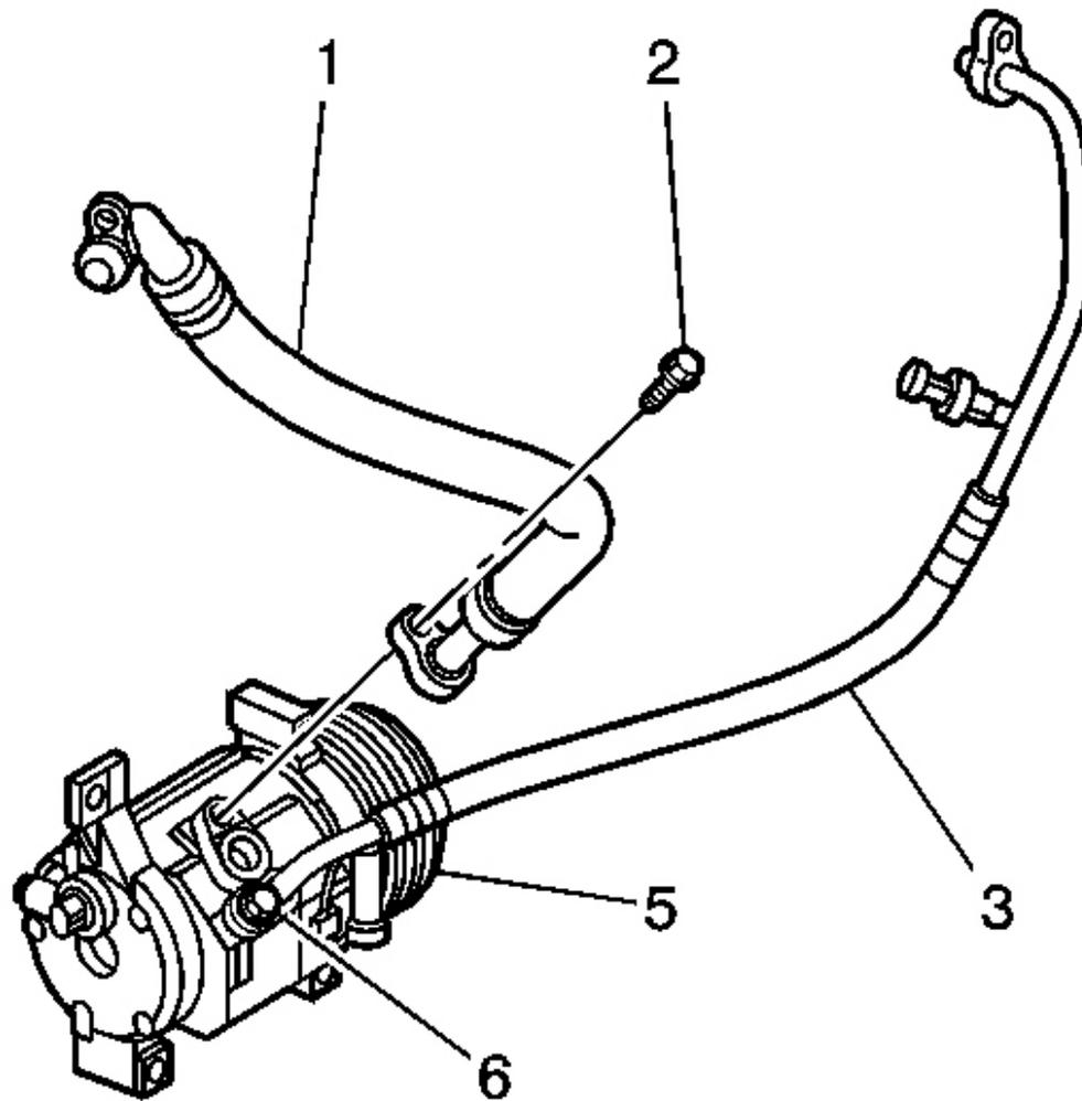
**Fig. 23: Discharge Hose & A/C Compressor**
