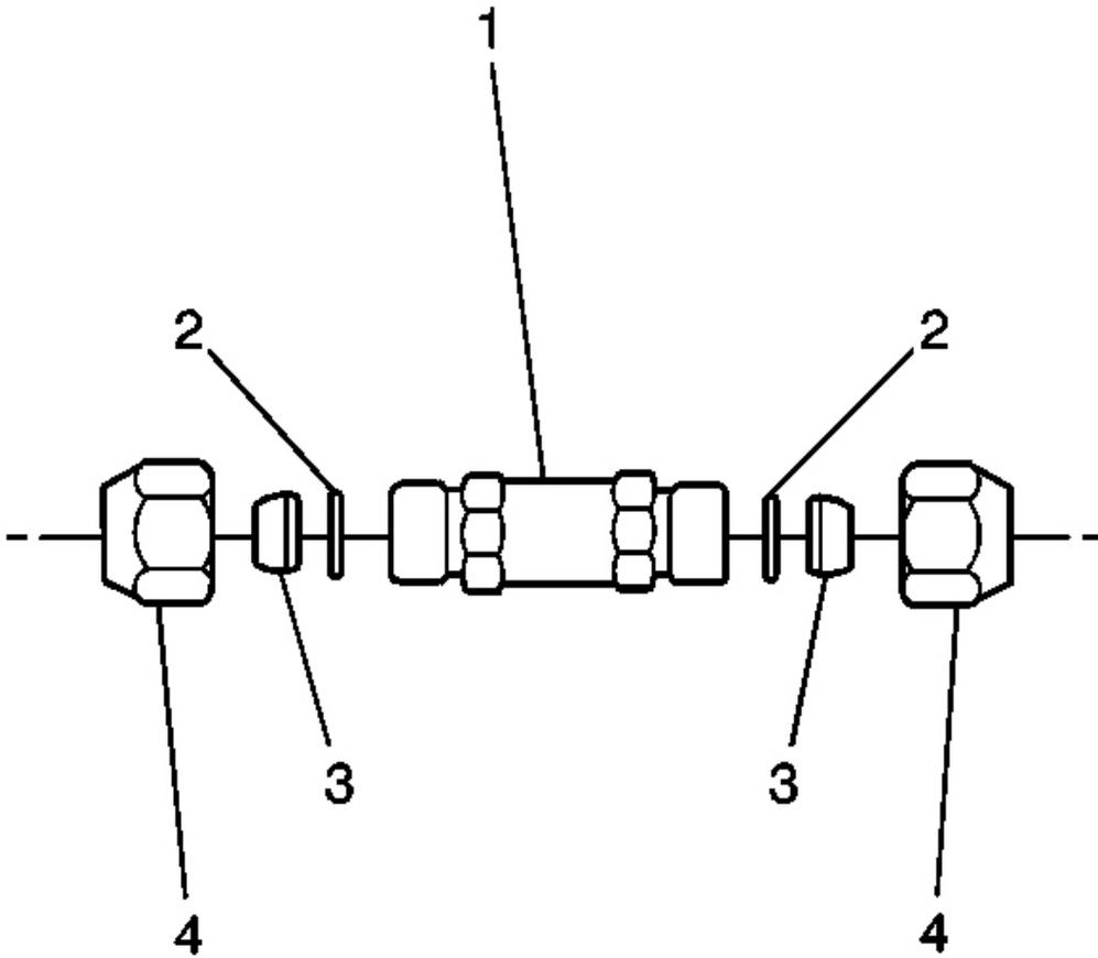
**Fig. 38: A/C Refrigerant Filter Components**
