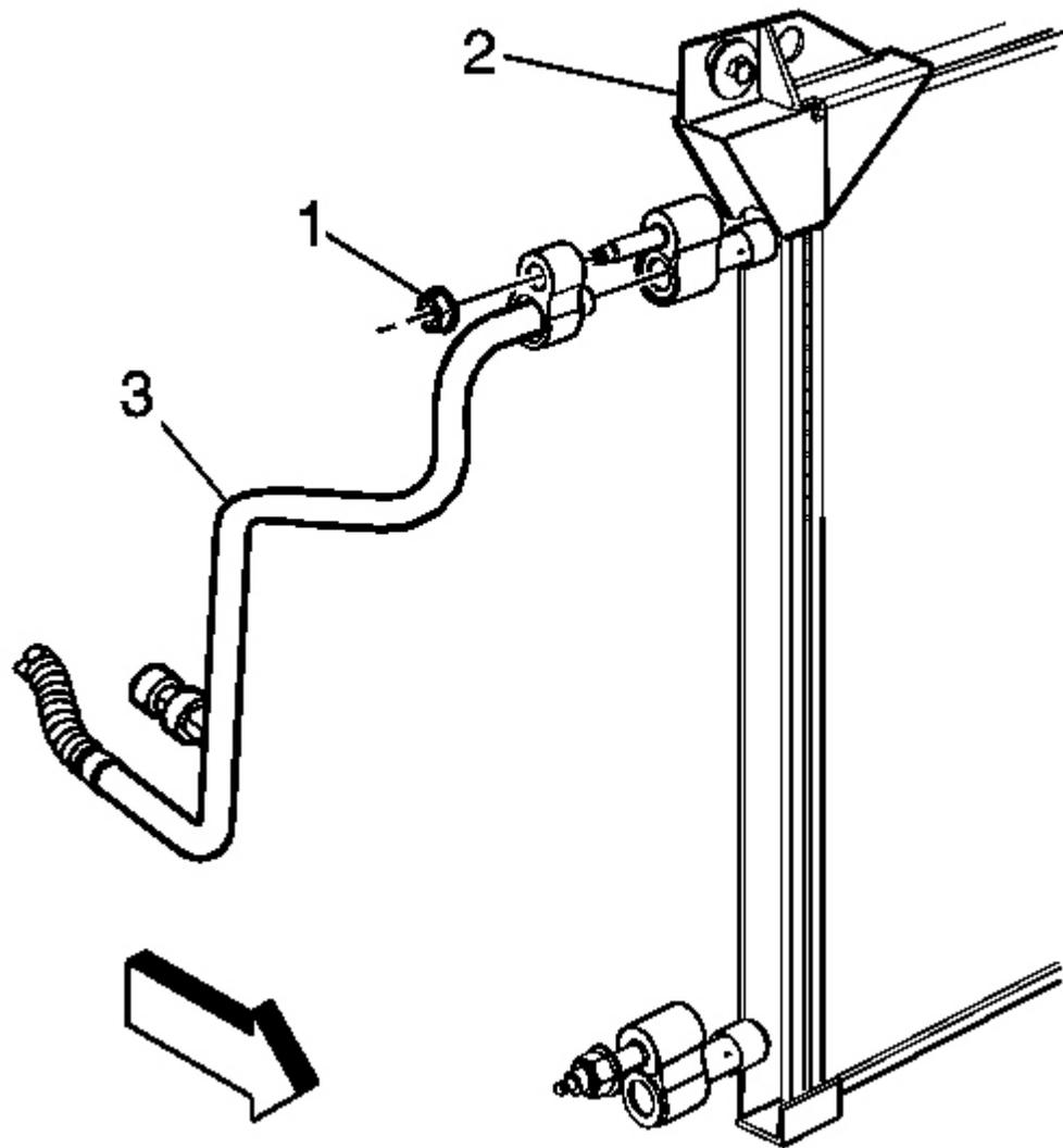
**Fig. 22: Discharge Hose Nut & Condenser**
