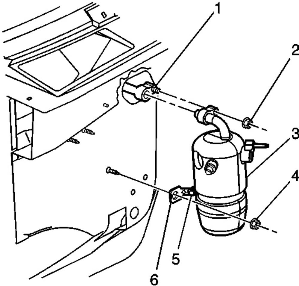
**Fig. 56: Retaining Bracket & Accumulator**
