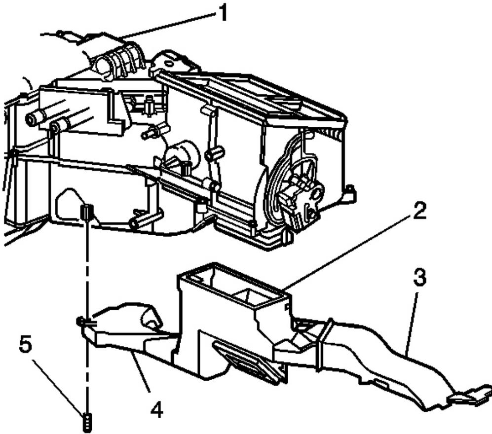
**Fig. 100: Floor Air Outlet Duct (LH)**
