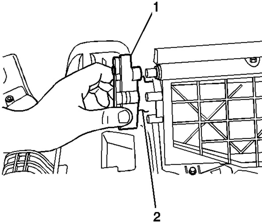
**Fig. 145: Recirculation Actuator And Recirculation Housing**
