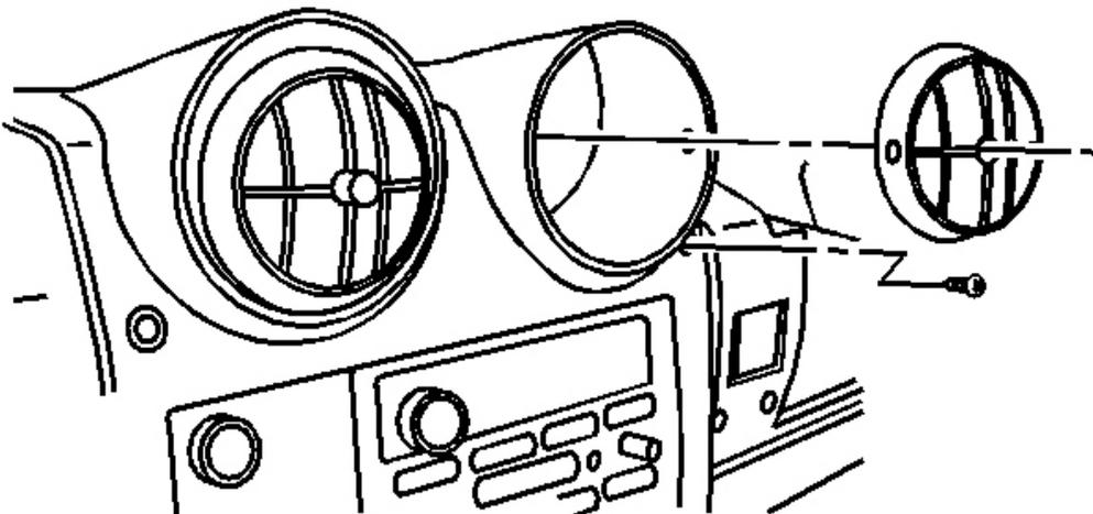
**Fig. 92: Air Deflector Louver & Instrument Panel (Center)**
