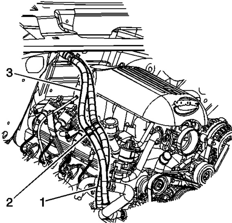
**Fig. 68: Heater Inlet Hose & Mounting Clip**
