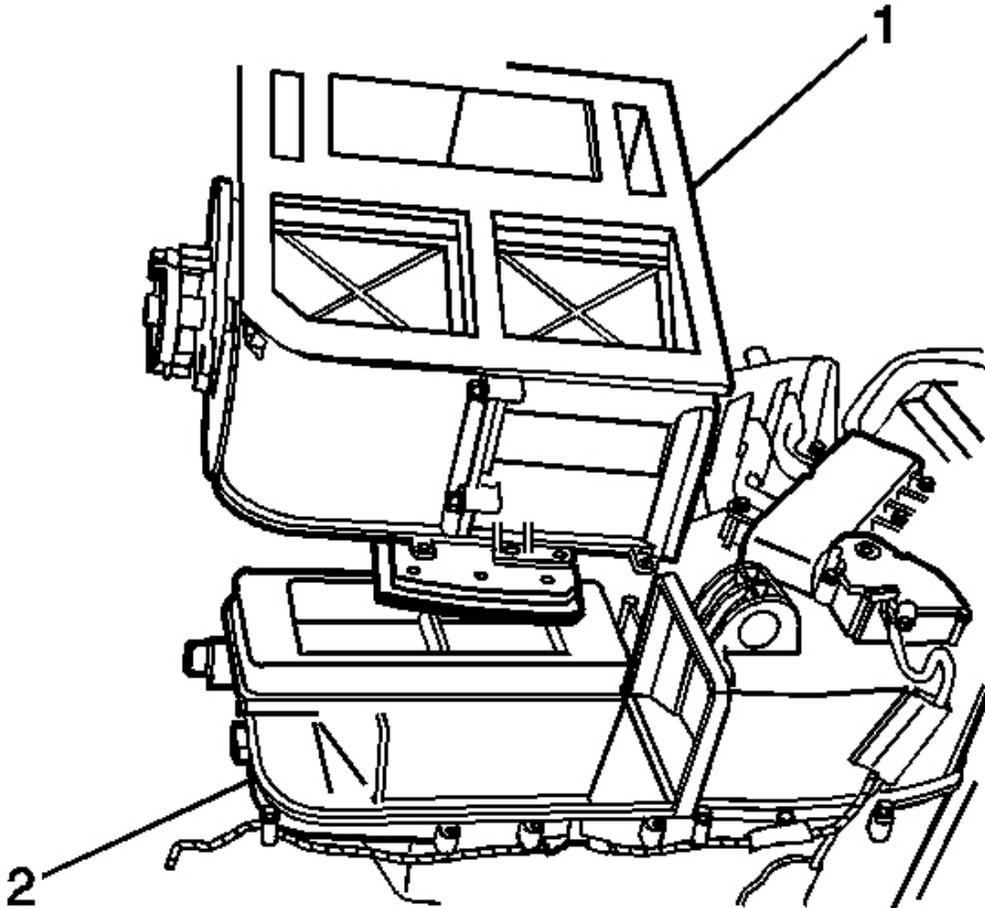
**Fig. 134: Air Distribution Housing And HVAC Module Assembly**
