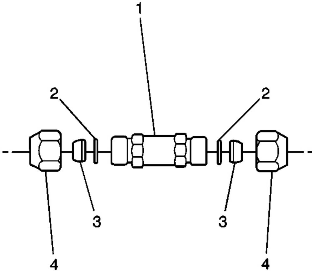
**Fig. 36: A/C Refrigerant Filter Components**
