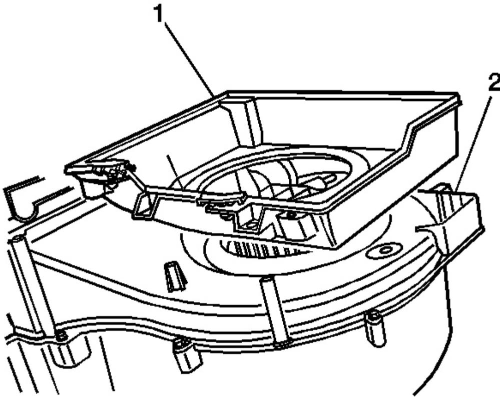
**Fig. 106: Lower Recirculation Housing**
