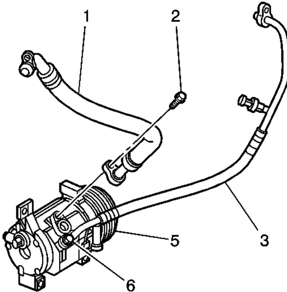
**Fig. 27: Discharge Hose & A/C Compressor**
