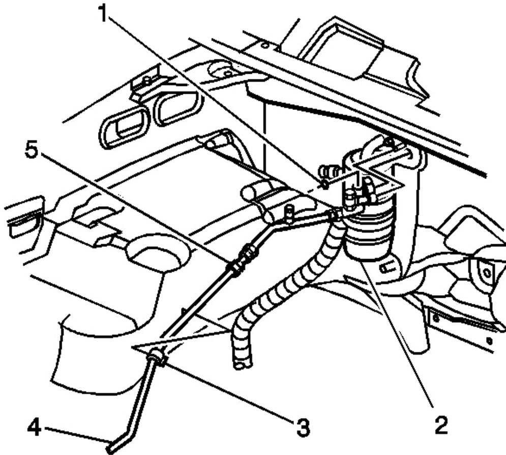
**Fig. 39: A/C Refrigerant Filter & Evaporator Tube**
