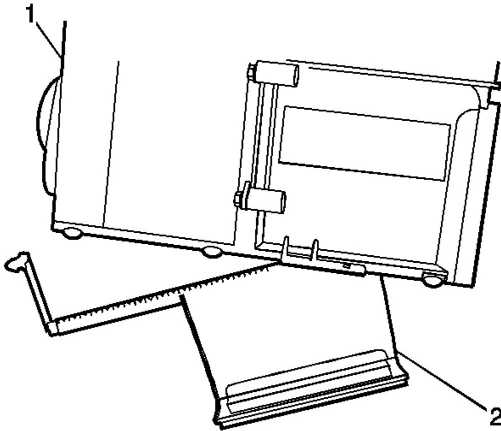
**Fig. 130: Lower Mode Door & Air Distribution Housing**
