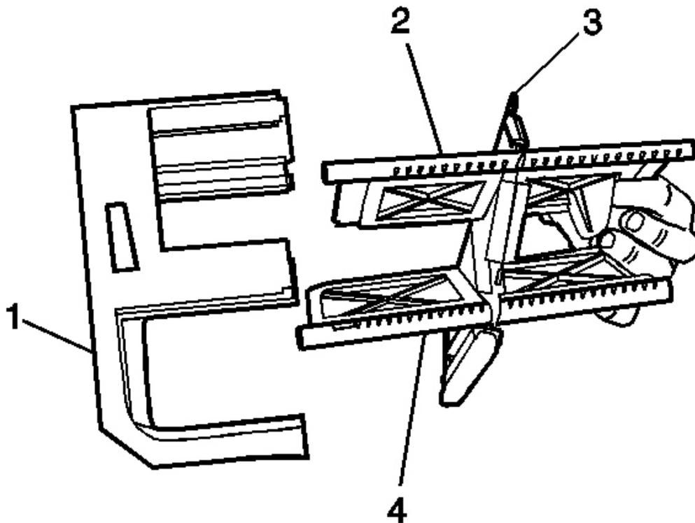
**Fig. 136: Upper Mode Door & Door Assembly**
