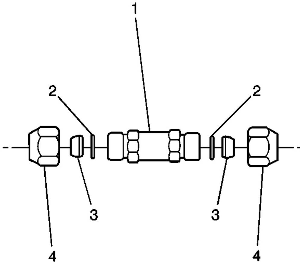
**Fig. 35: A/C Refrigerant Filter Components**
