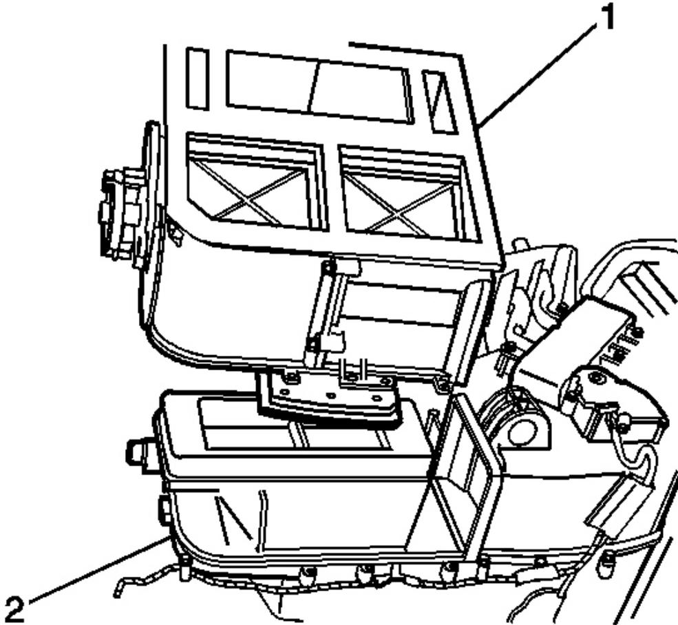
**Fig. 116: Air Distribution Housing And HVAC Module Assembly**
