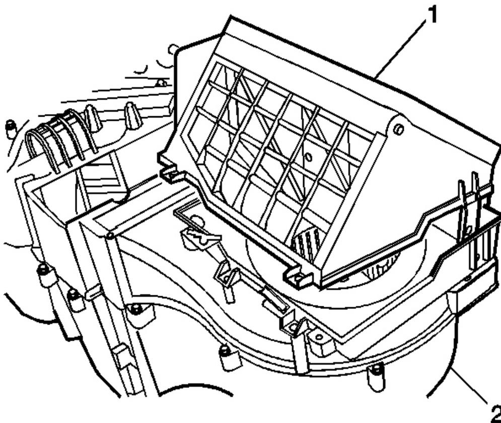
**Fig. 141: Air Distribution Housing And HVAC Module**
