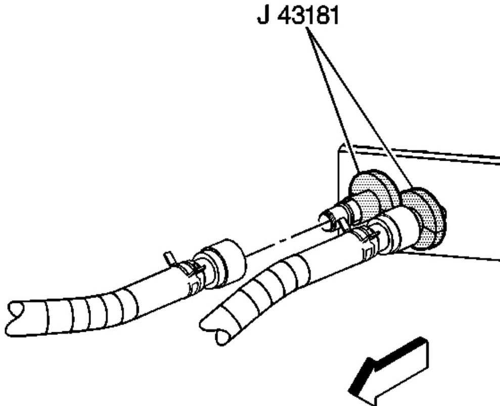
**Fig. 67: Identifying Heater Hose To Heater Core Outlet**
