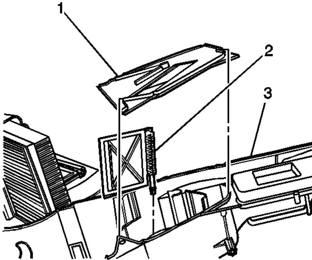
**Fig. 120: Left Temperature Door & Lower HVAC Module Case**
