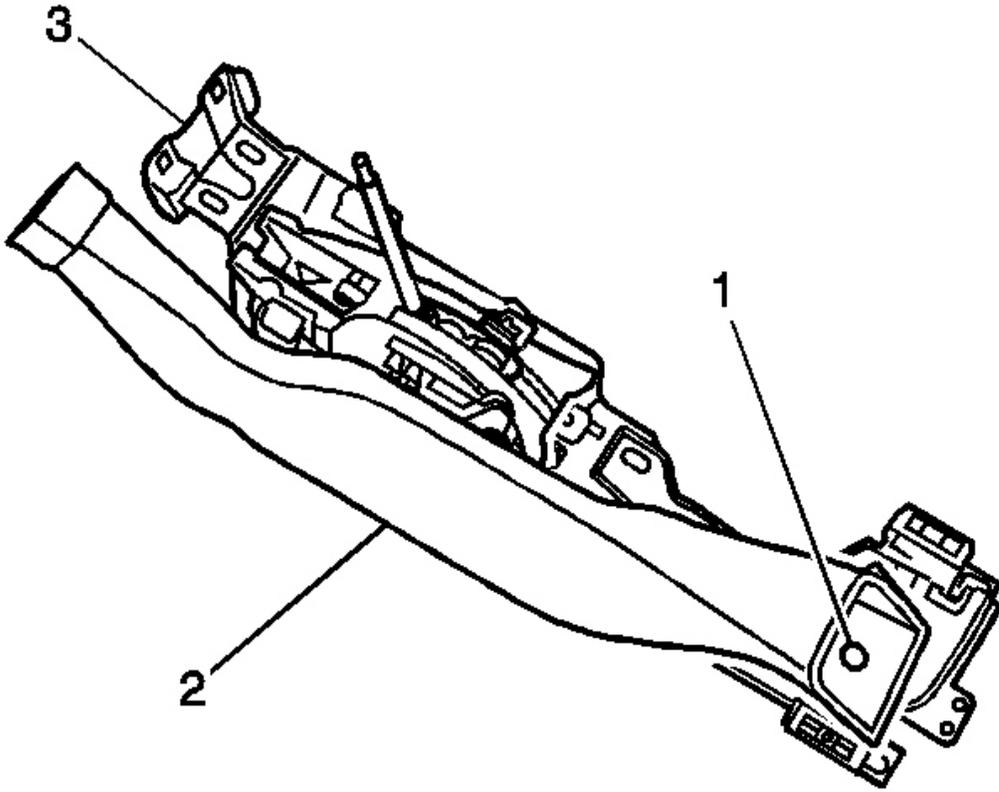
**Fig. 95: Identifying Push Pin (Rear Floor)**
