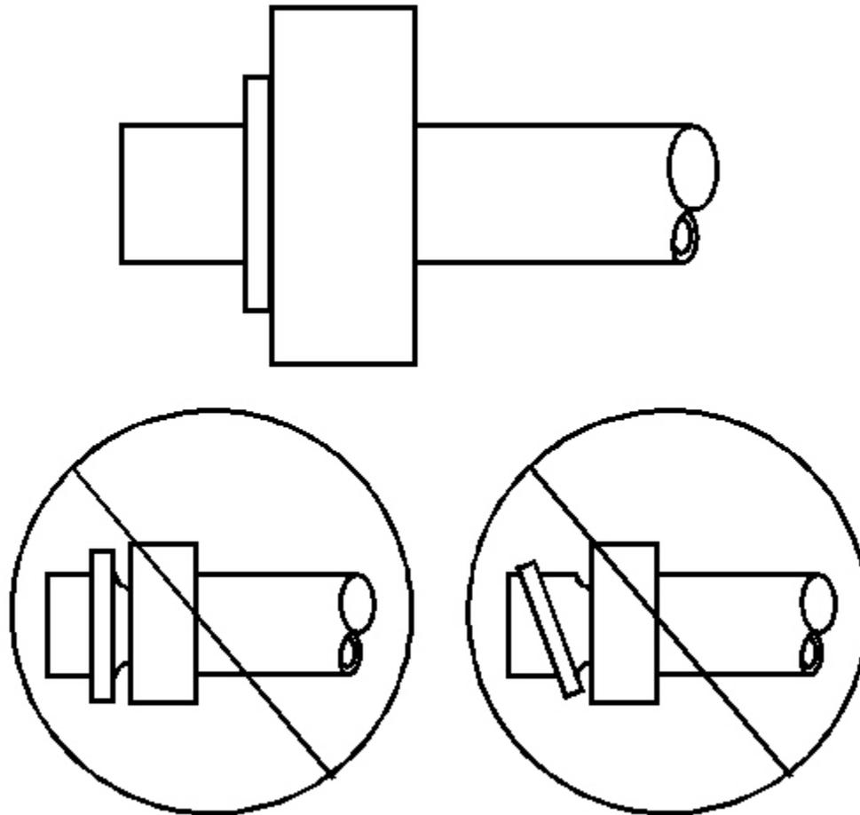
**Fig. 16: Identifying Sealing Washer**
