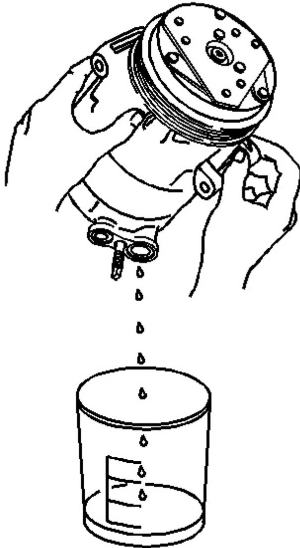
**Fig. 4: Draining A/C Compressor Oil**
