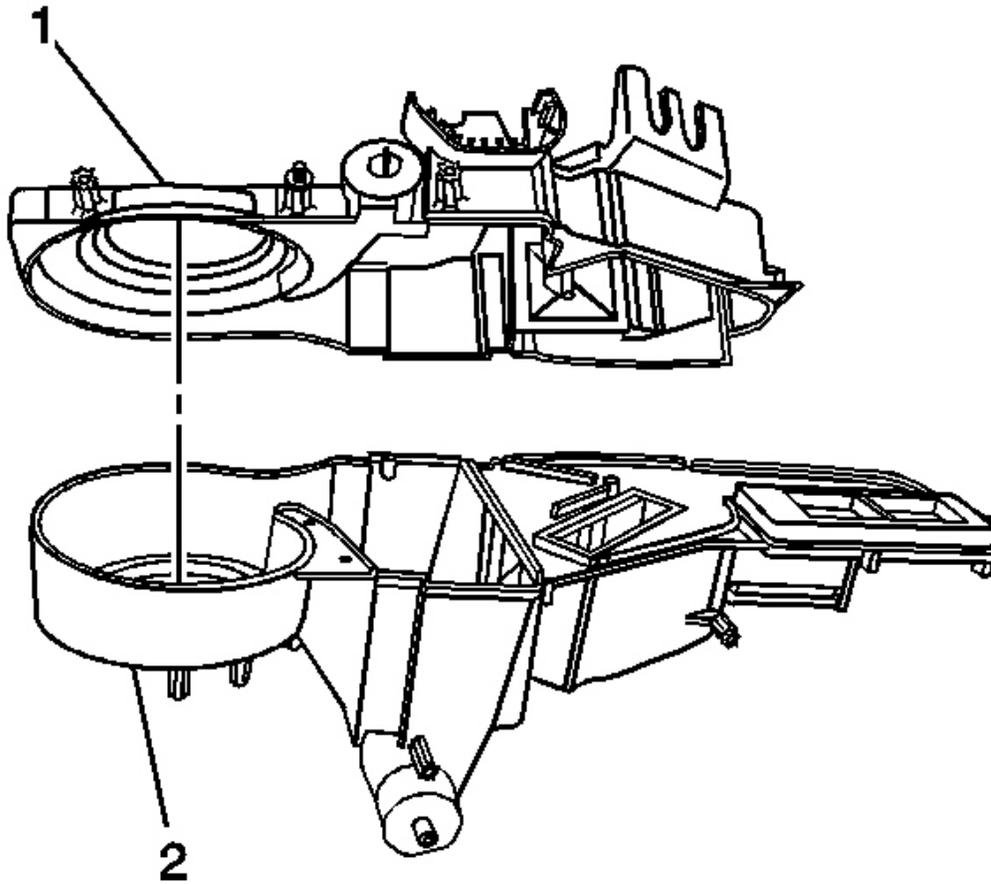
**Fig. 107: Upper HVAC Module Case And Lower HVAC Module Case**
