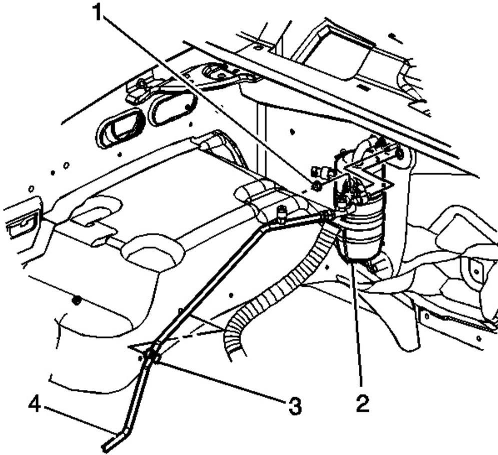
**Fig. 29: Evaporator Tube Nut & Evaporator**
