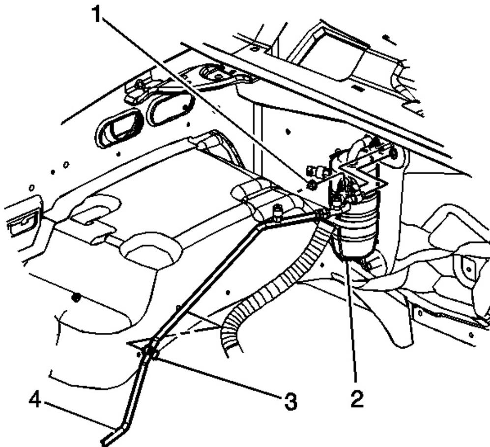
**Fig. 30: Evaporator Tube Nut & Evaporator**
