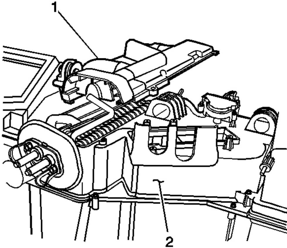
**Fig. 66: Evaporator Cover & HVAC Module**
