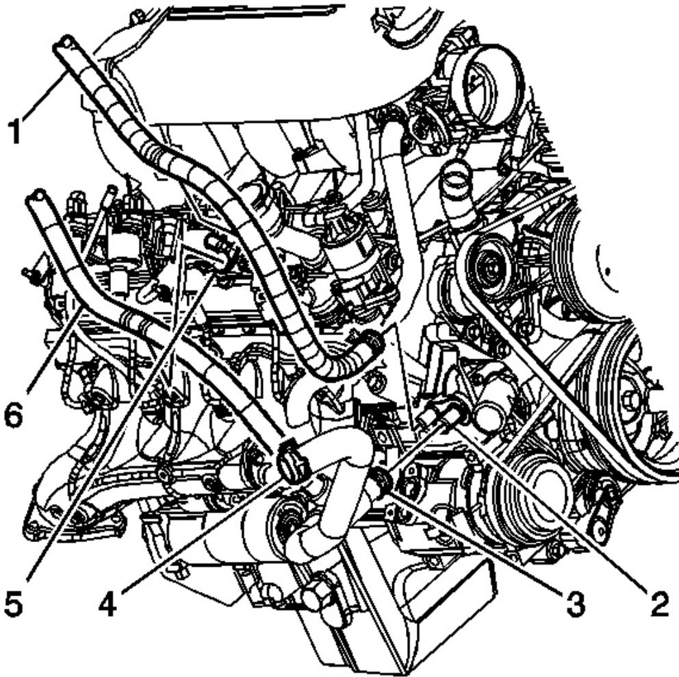
**Fig. 69: Heater Inlet Hose & Engine**
