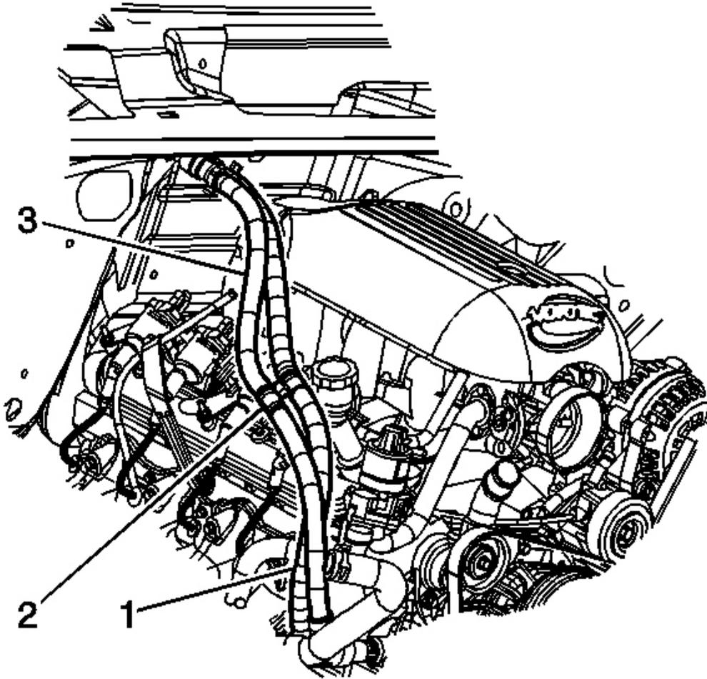
**Fig. 74: Heater Inlet Hose & Mounting Clip**
