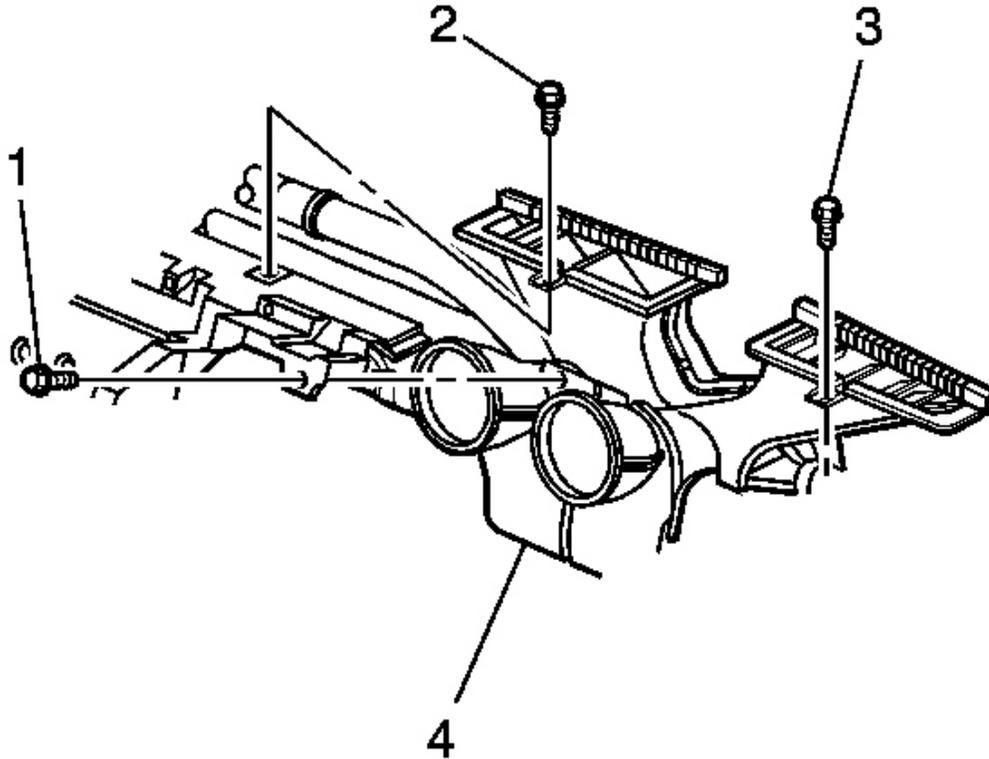
**Fig. 88: Screw & Air Distribution Duct**
