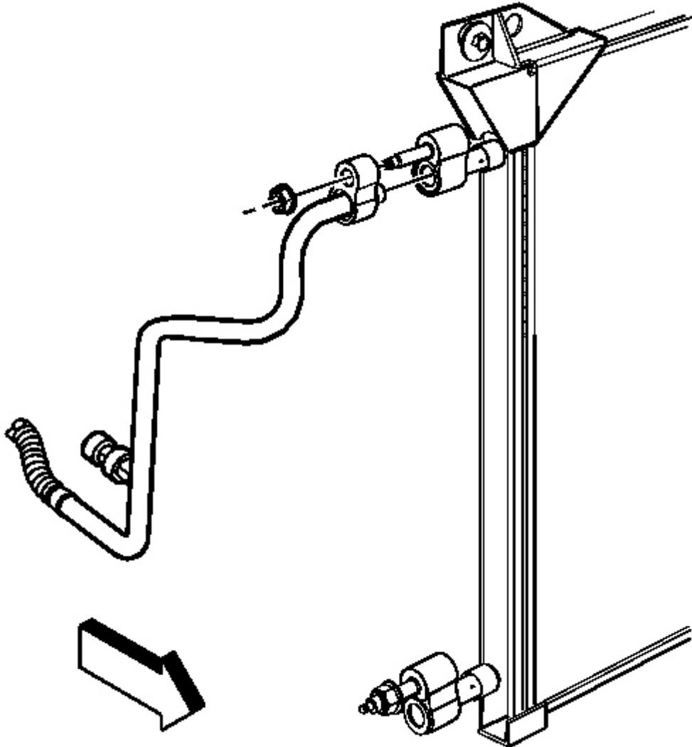
**Fig. 48: A/C Refrigerant Pressure Sensor & Evaporator Tube**
