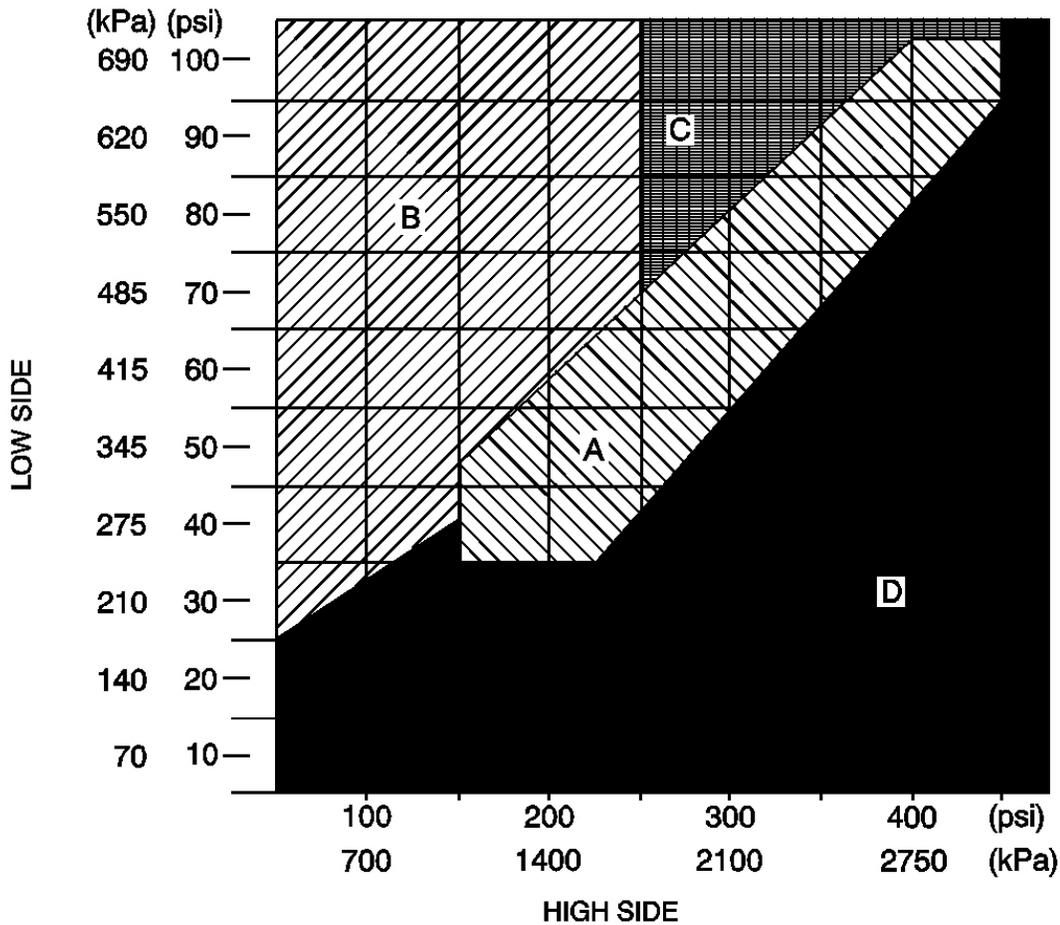
**Fig. 1: A/C System Pressure - Zone Classification**
