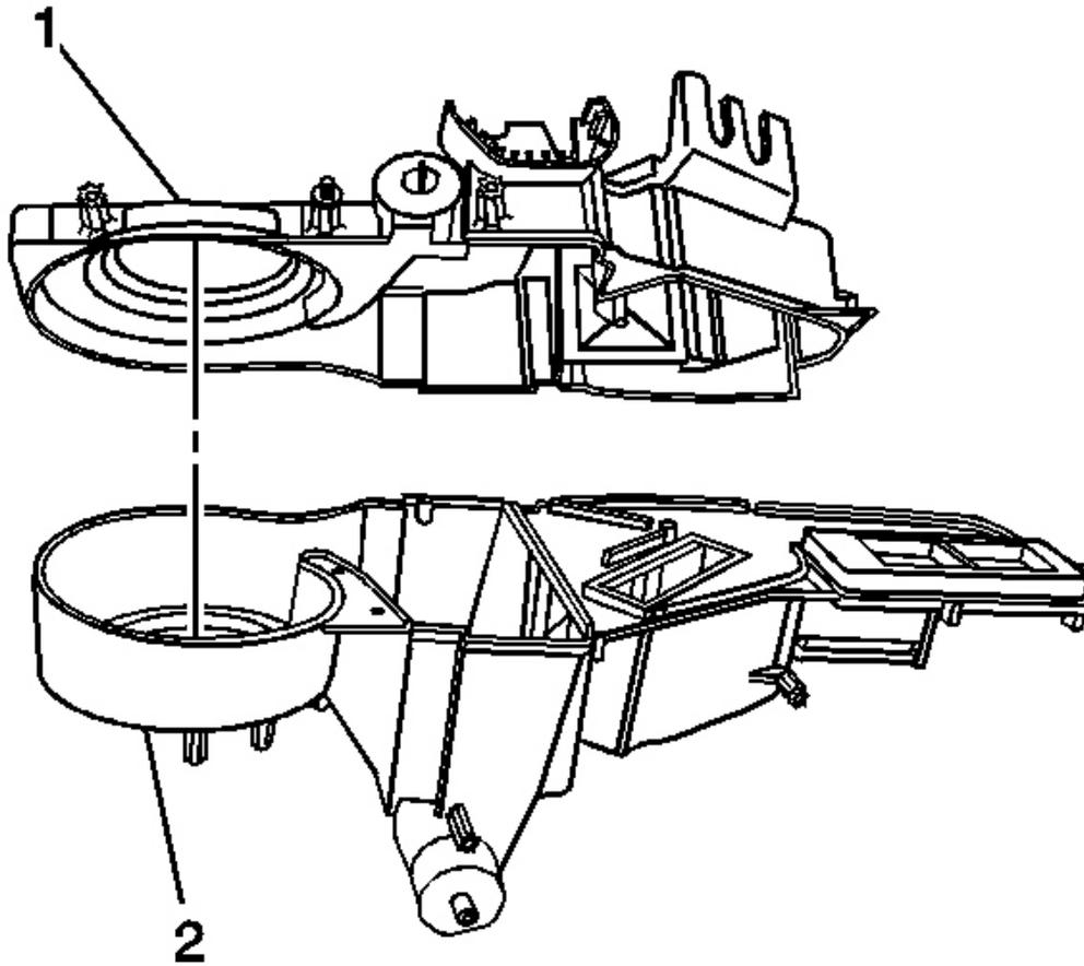
**Fig. 119: Upper HVAC Module Case And Lower HVAC Module Case**
