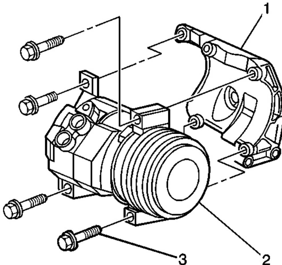
**Fig. 6: A/C Compressor Mounting Bolts (L18)**
