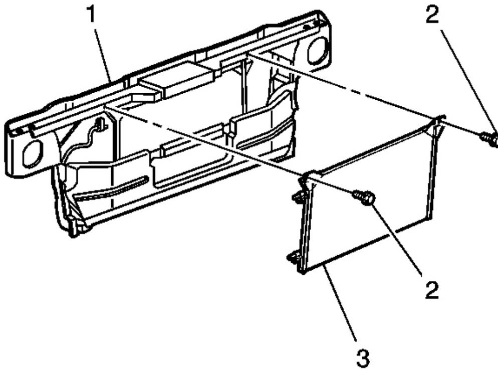
**Fig. 51: Condenser & Mounting Bolts**
